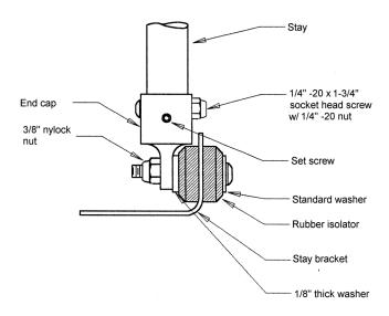
Fig. 5 Stay mounting bracket assembly.
