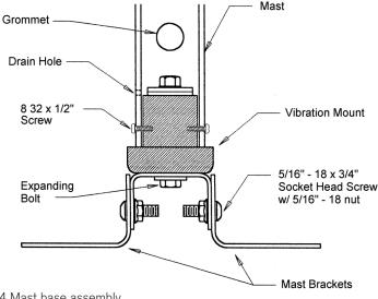
Fig. 4 Mast base assembly.
