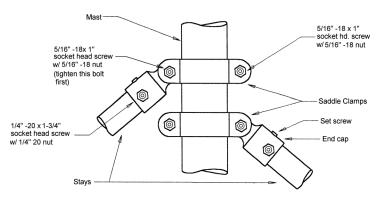
Fig. 3 Saddle clamp, end cap and stay assembly.
